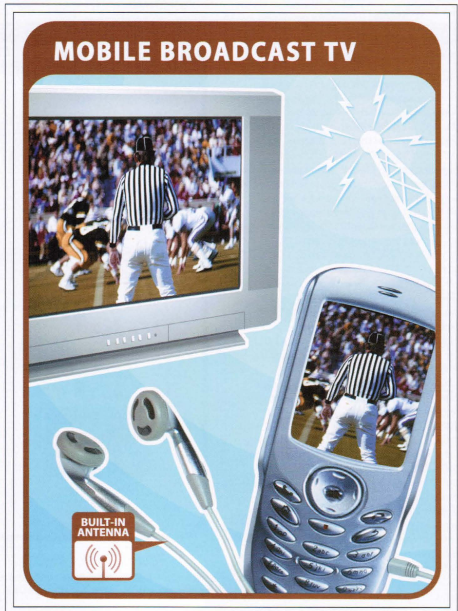
Fig. 2: To increase antenna size, mobile TVs are generally built with antennas integrated into a lanyard or special headphone leads – a solution with its own problems.
